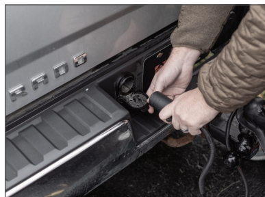
Vehicle power connection to eliminate hand cranking and RV battery drain
